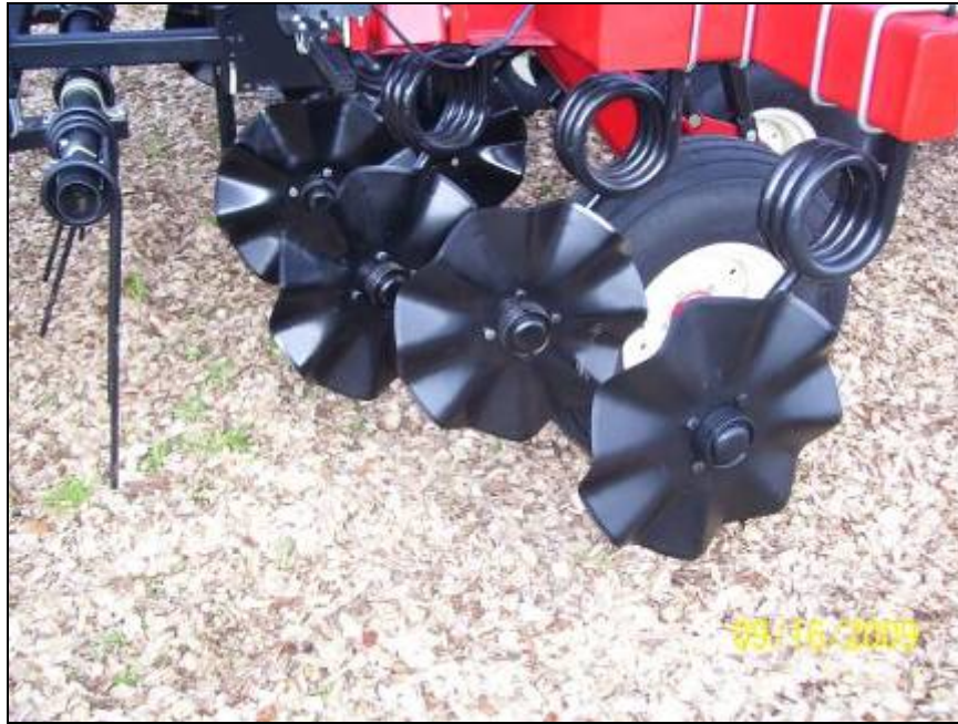
Figure 2. An 8-wave fluted blade on a vertical tillage implement manufactured by Salford. Note that the blades are spring-mounted and that this implement has harrow tines.
