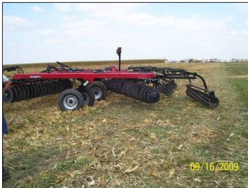
Figure 1. One example of a vertical tillage implement, the Case True Tandem 330. Photo taken at Husker Harvest Days in fall 2009.
